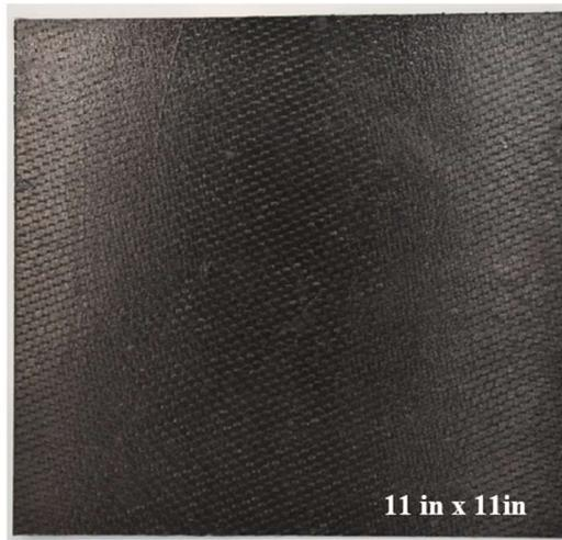
Figure 4. A CF/UHTR 2D laminate sample (11 inches by 11 inches by 0.1 inches).
