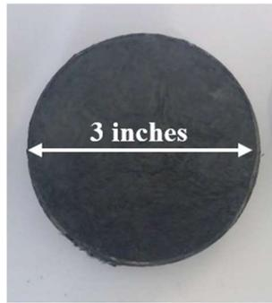
Figure 3. A CF/UHTR MC sample (3 inches in diameter and 0.5 inch in thickness).
