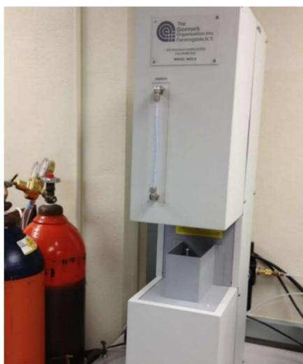
**Figure 6. Microscale Combustion Calorimeter (MCC-2) by Govmark Organization Inc.**
