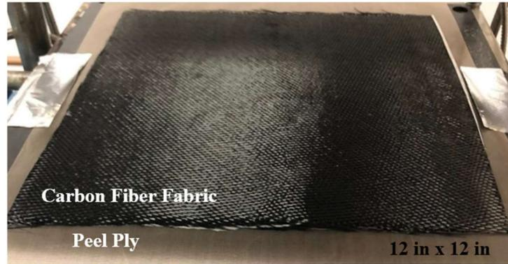
Figure 1. Pre-cut carbon fiber mat (12 inches by 12 inches) laid on a hot press pre-heated at 150°C).
