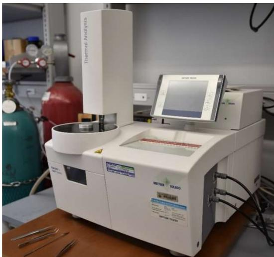
**Figure 5. Thermogravimetric Analyzer (TGA/DSC 1 S STAR<sup>®</sup> System) by Mettler Toledo.**
