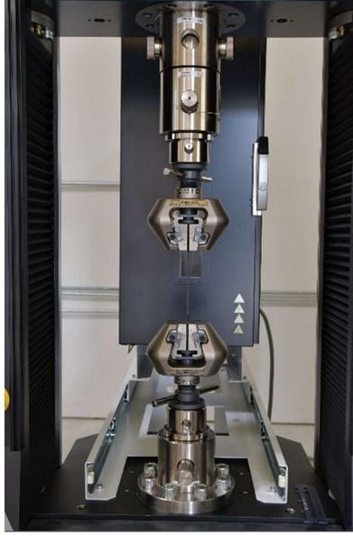
**Figure 8. Shimadzu Universal Testing Machine: Tensile testing set-up.**
