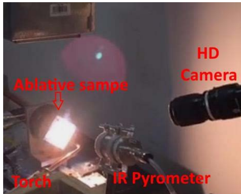
Figure 4. Overview of the ablative testing setup [3].
